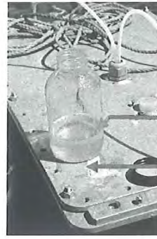
Figure 7 Sample Taken During series No.2, Presence of an Emulsion at the Water Surface
